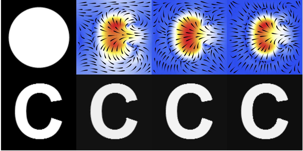
**Fig. 1.** The mapping of a circle (top left) onto the letter “C” (bottom left) with classical fluid registration equation (1) (second column,  $(\mu, \lambda) = (5/2, 0)$ ), the fluid diffusion equation (17) (third column,  $\alpha = 1024$ ) and fluid optical flow equation (17) (last column  $\alpha = 1024$ )
